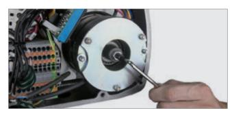
Adjusting clutch torque, if necessary, is convenient with an Allen key tool.  $\blacktriangle$
