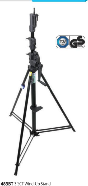
w/Auto Self-Locking Device Black 3 sections. Dia.: 55mm, 45mm, 38mm. Leg dia.: 30mm. 2 risers extend simultaneously at one elevation of 4.4cm per handle turn.
