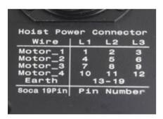
Wiring information clearly disclosed on the front panel (for 8-CH controller) in favor of the user making the corresponding cable assembly for chain hoist controlling system.
