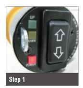
Once chain hoist power is connected the power LED indicator will on. Let you know the motor is ready to go.
