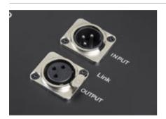
Built up with 3-PIN XLR in/out connector as linkable ports for multiple system.
