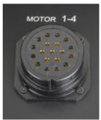
Industry standard connectors: power input 32A 5P CEE receptacle; output 16A 4P CEE (4-CH) or 2 x 19-PIN connectors (8-CH). Four or eight channels of direct control using reversing contactors built on the rear side of the panel.
