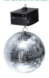
Apart from conventional one. DMX mirror ball motor offers a flexible and selective control for the rotation. and generates much more diverse effects. It is compatible with standard DMX-512, and runs for 2 channels. The metal chassis is compact and sturdy, and also comes with a M10 fixing hole on top of bracket which makes installation easy and fast. It is designed to fit wide range of mirror ball size up to diameter 50 cm.
