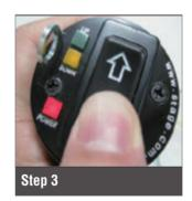
Down direction with Yellow LED indicator to tell correct operation way even in dark.
