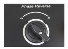
Phase reverse switch helps to convert the phase into correct sequence.
