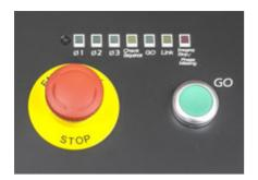
Phase check for clear identification of respective incoming phases. Only when the phase sequence is correct does the equipment start to work. Phase missing displays on a red LED indicator and the quipment won't be functioning. Lockable E-Stop button and phase reverse switch as standard feature.
