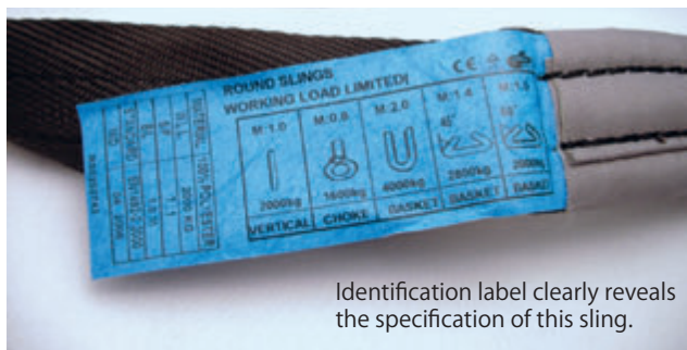
Visible two black lines stands for load capacity of 2,000kgs.
