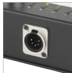
5-pin XLR to communicate with main controller.
