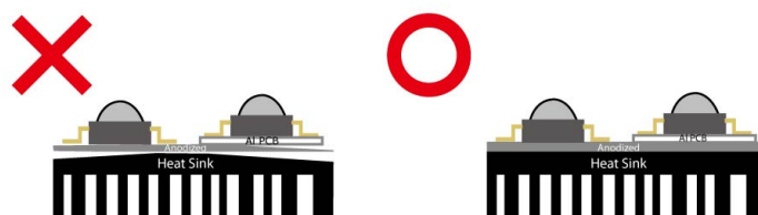
<Figure 22 Edixeon ® ARC series assemble with heatsink>
