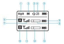
Home screen: If no operation is performed for 20 seconds on the other screens, the display will automatically return to the home screen.
