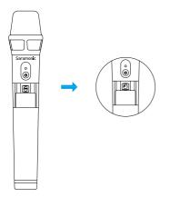
4. The system is paired successfully when the indicators of the RX and HU turn solid blue.
