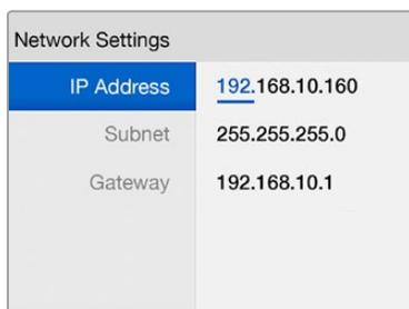
Use the rotary knob or the view buttons on Blackmagic MultiView 16's control panel to assign values to your network settings.
