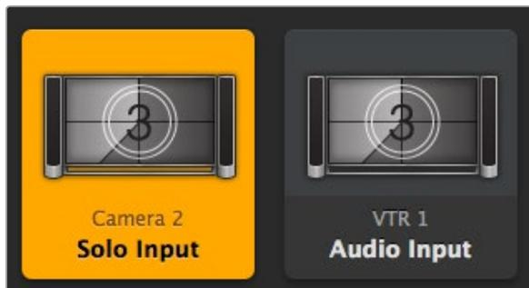
The "solo input" and "audio input" pushbuttons allow you to change the corresponding Blackmagic MultiView 16 settings using Videohub Control.
