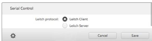
Select either 'client' or 'server' when using RS-422 serial control.
