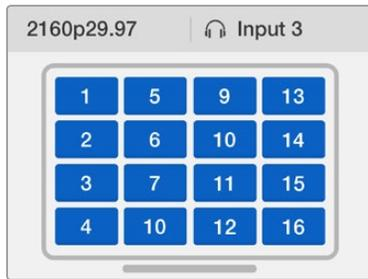
The 'home' screen is the default display on Blackmagic MultiView 16's control panel LCD. This screen displays your selected multi view layout, the frame rate for the multi view SDI output, and the selected SDI input used to embed audio into the multi view output.
