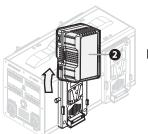
Remove all the battery packs, there should be no packs on V mount plate.
