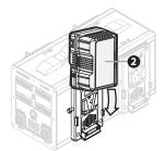
(02) Connect at least one battery pack on 4 V-mount plates.
