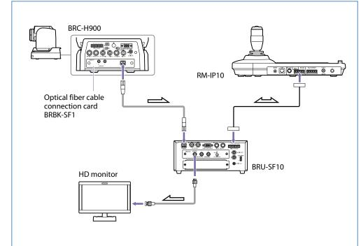
Video signal: Optical Fiber Cable CCFC-S200 Video signal: Connecting cable with BNC connector Remote control signal: Network cable modified for terminal block connection (Cat 5e or higher) Signal flow
