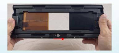
Adjust the lock to the unlocked position.
