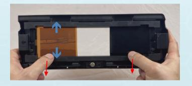
2. Push the Lower Magnetic Film Guide gently downwards until the 120 Film is fully extended.
