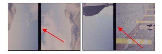
Based on the above image, the misalignment issue causes incomplete presentation of the photographs and also results in the XA+(or XAs) scanner capturing the inter-frame space (indicated by the red arrow in the image).
