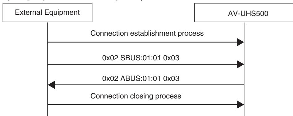
Example; Crosspoint (XPT) control of the buses (Error; Out of the parameter range)
