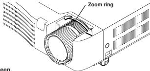
**2** Adjust the projection image to the screen. Check that the screen is set level and vertically.
