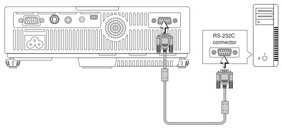
Serial cable (D-Sub 9-pin, straight) (commercially available)
