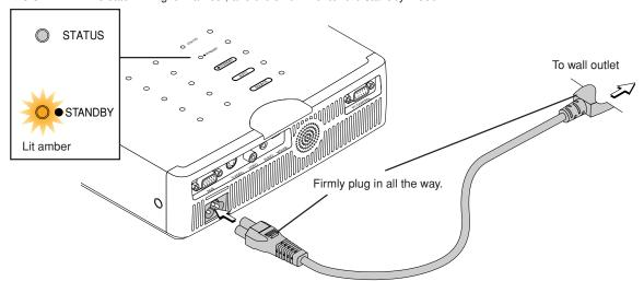
**2** Switch on the projector power Press the STANDBY button.
